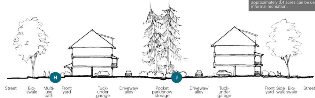
A section drawing that cuts through the center of a block shows how informal open space that doubles as snow storage in the winter fits between buildings.
