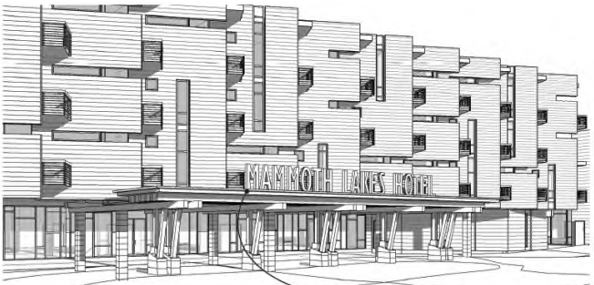
Lighted Monumental Signage: Metal Letters Mounted to Steel Armature
