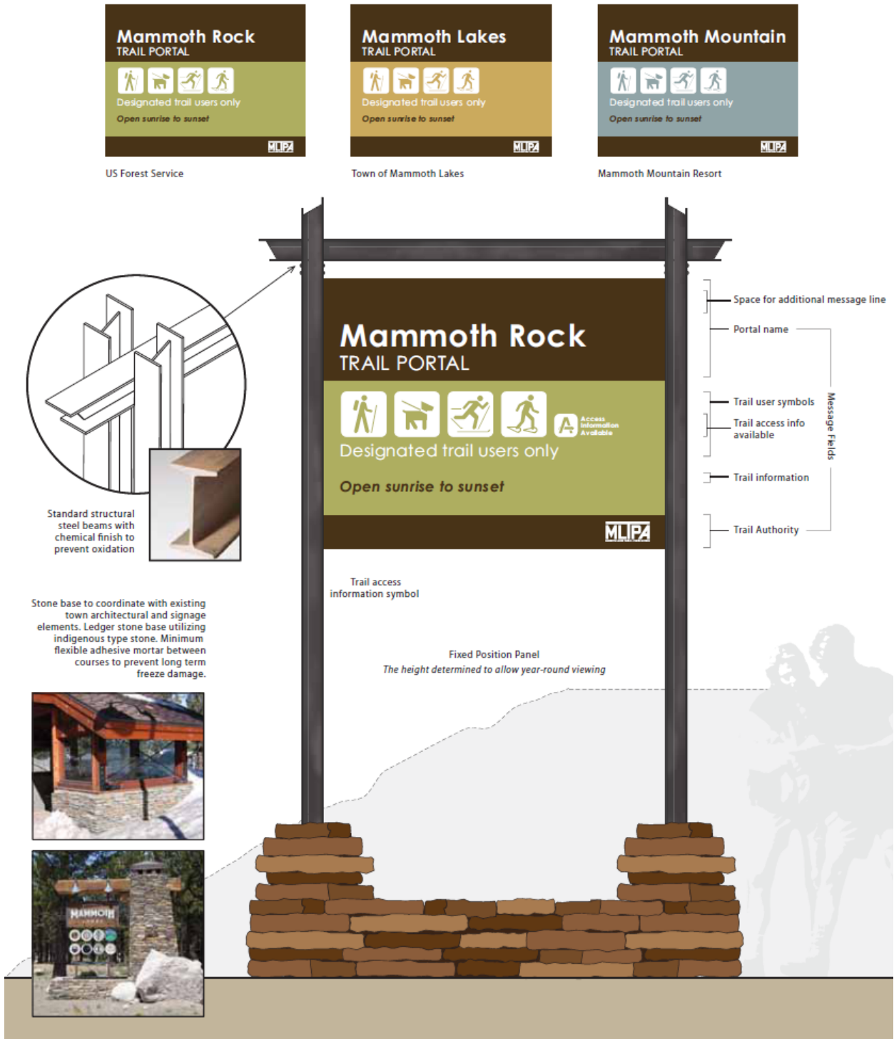
Figure 5-13. Portal Identification Marker
