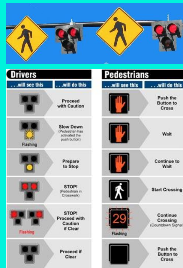
Figure 5.20 High-intensity Activated Crosswalks (HAWK Signals)
