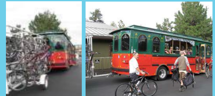
Figure 1.8 The majority of the trolleys in Mammoth Lakes on fixed lines are equipped with a bicycle rack that can accommodate three bicycles. The Lakes Basin trolley is equipped with a trailer and can hold a total of 22 bicycles.
