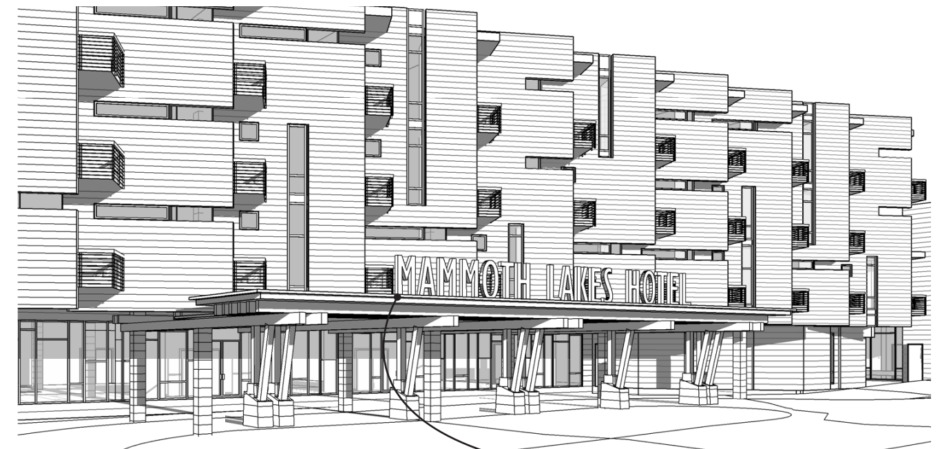
(C) 3D View of Hotel Signage Lighted Monumental Signage: Metal Letters Mounted to Steel Armature
