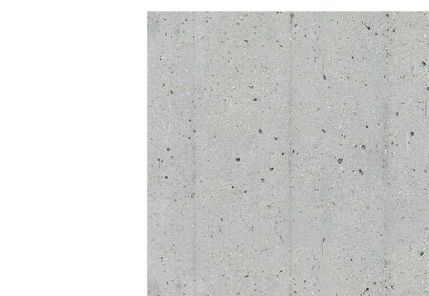
(CONC) CONCRETE - ARCHITECTURAL CAST-IN-PLACE
