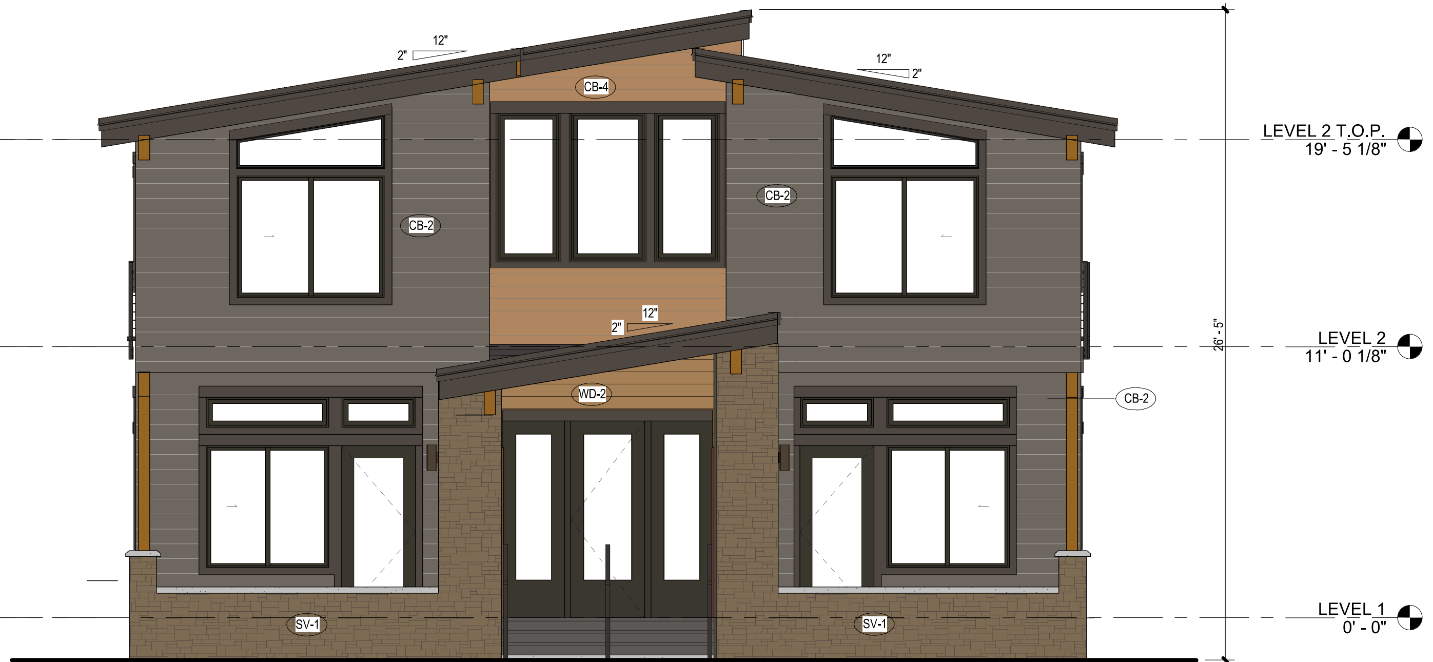
FRONT ELEVATION SCALE: 1/4" = 1'-0"
